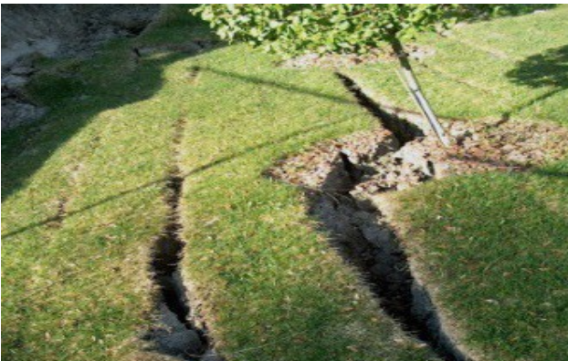
Figure 5 Tension cracks may indicate a pending slope failure.
